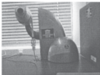
Fig. 1: (a) A photo and (b) a schematic overview of the FOT standard setup. Legend: LS - loudspeaker; BT - bias-tube; PN - pneumotachograph; PT1 and PT2 - pressure transducers; bf - biological filter with mouthpiece; nc - nose clip to prevent leakage of air-flow via the nose; R_q - known resistance in the pneumotachograph used to calculate flow; Q(t) - flow; P(t) - pressure; U_g(t) - multisine input generated using a loudspeaker (LS)
